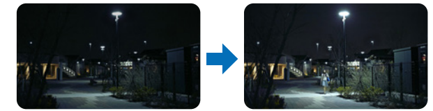
Illuminate brightly enough not only directly under, but also a short way ahead of a passerby
